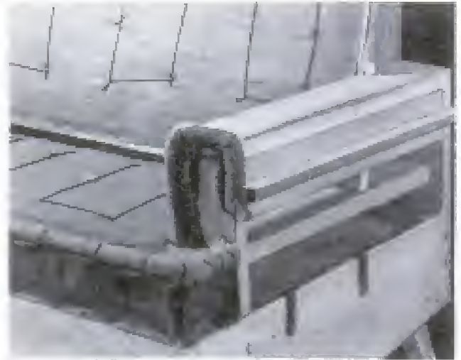
Above, close-up view of arm and corner of seat show how edge roll should look. Roll is tacked to arm and sewed to seat. Long stitches fasten burlap to springs
